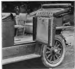
The extra seats in this Locomobile phaeton may be made to face in two directions.
